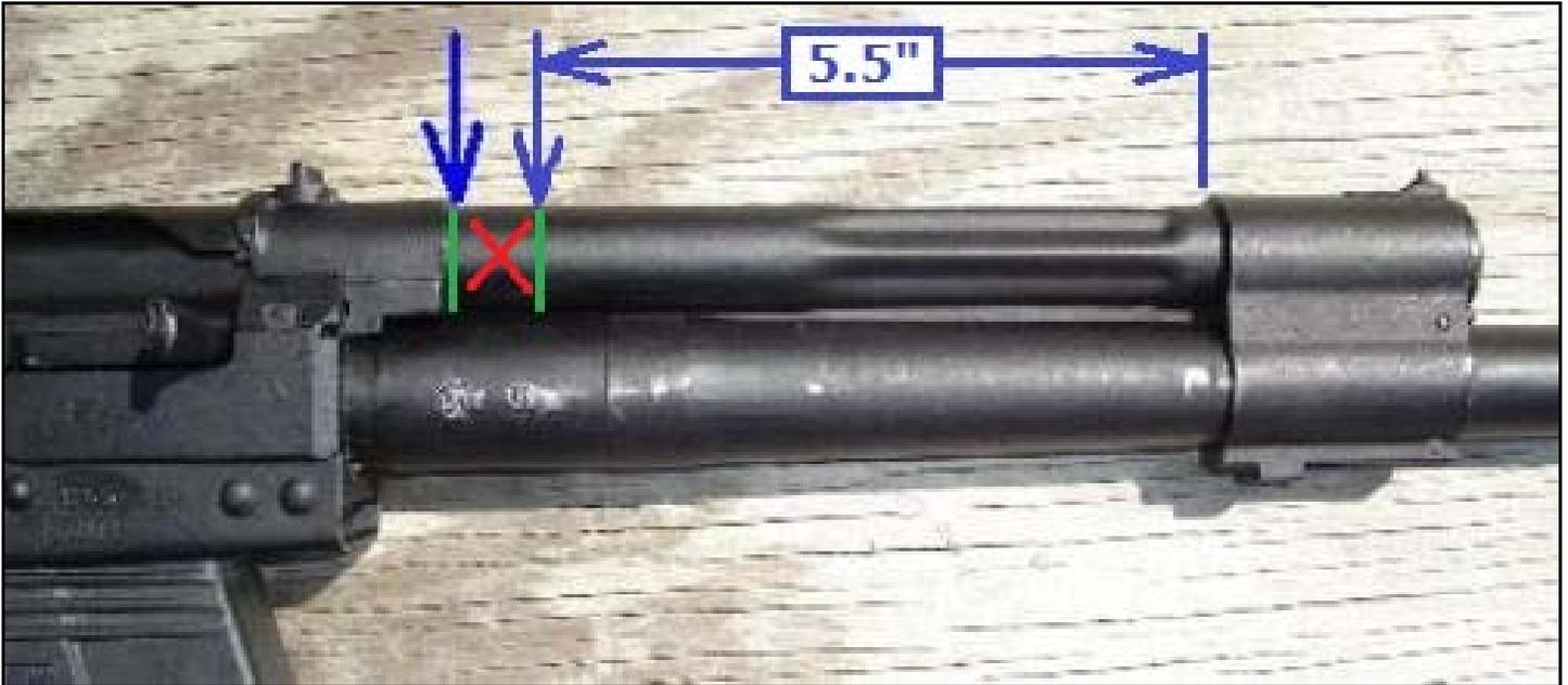
\*If you are cutting the tube, measure 5.5" back from the gas block and mark the tube with a pencil. Cut through the tube at that mark and again immediately in front of the rear casting that engages the front of the receiver. This will give you enough clearance to remove the 2 pieces. Use a hack saw or an abrasive chop saw.
