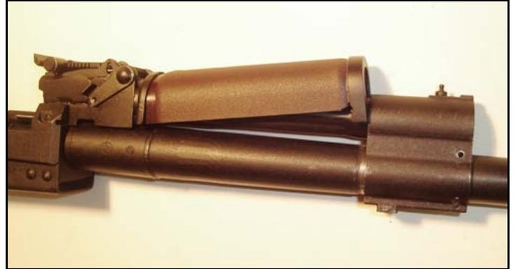
\*Install the upper handguard by sliding the back end into the rear upper retainer on the tube and sliding the upper front retainer on to handguard and rotate down into place.
