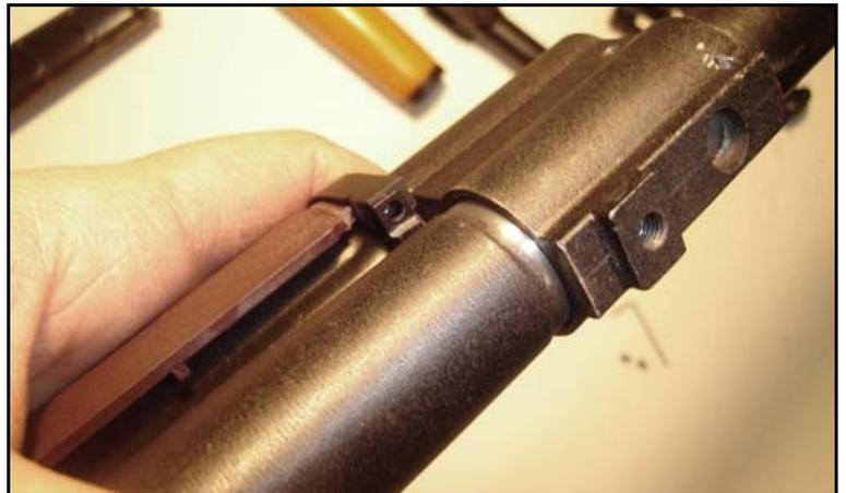
\*Slide the front upper retainer keeper between the barrel and gas tube and attach with screws.
