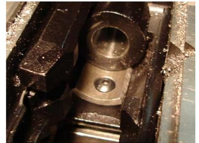
Should you see or feel the tap flexing, back it off to break the chips and resume tapping. Sometimes you need to rock it back & forth to break all the chips. Do not flex the tap!!! Use a cutting fluid for best results.
