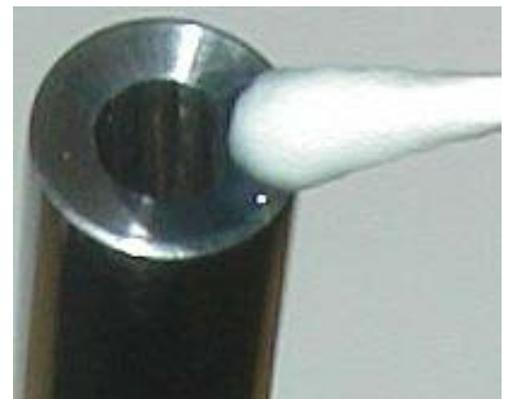
Degrease the muzzle with alcohol, then apply a bluing agent to the bare metal. OXPHO-BLUE, B/C Perma Blue, B/C Presto Pen or other bluing agent should be used to protect the freshly cut muzzle.
