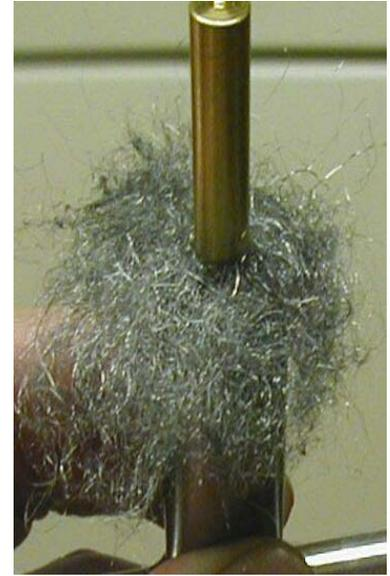
The finishing cut is performed with increasingly lighter pressure as cutting progresses until almost only the weight of tool is applied to the muzzle.
