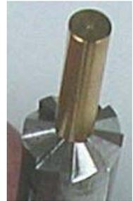
Required tools are the cutter, pilot, adapter or handle and a hex key. I recommend using a drill adapter rather than a handle. I have found you get a more consistent cut with this method. **DO NOT EXCEED 250RPM or side load the cutter, you will ruin the tool, bend the pilot, cause chatter marks on the muzzle and chew up your rifling!**
