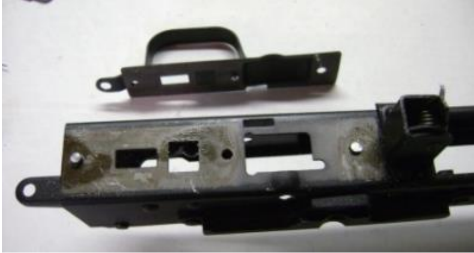
Receiver with bottom plate/triggerguard removed
