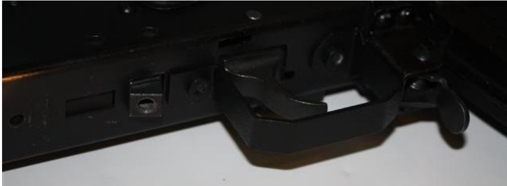
Painted receiver with fcg, triggerguard and pistol grip nut installed
